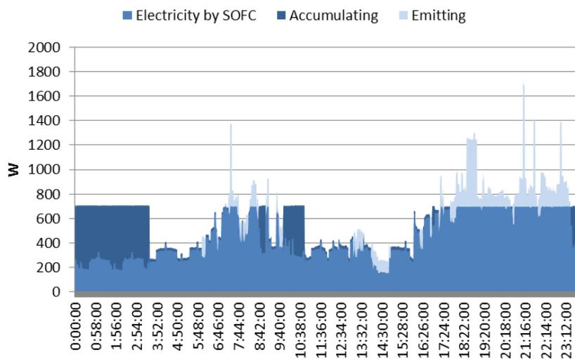
Figure 7: Supply of electric power (medium load)
