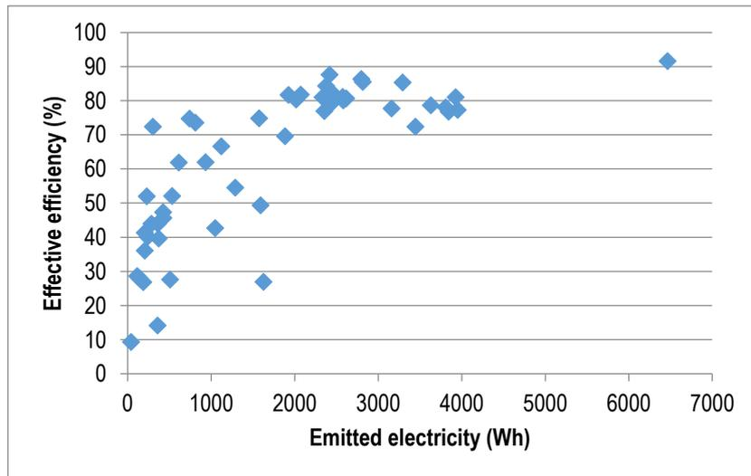
Figure 12: Battery's trait (effective efficiency vs emission)
