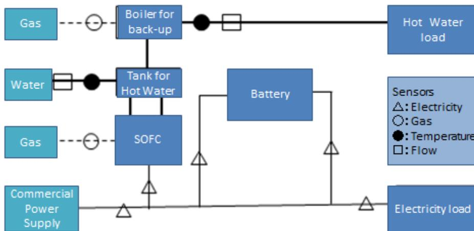
Figure 3: System of SOFC and battery
