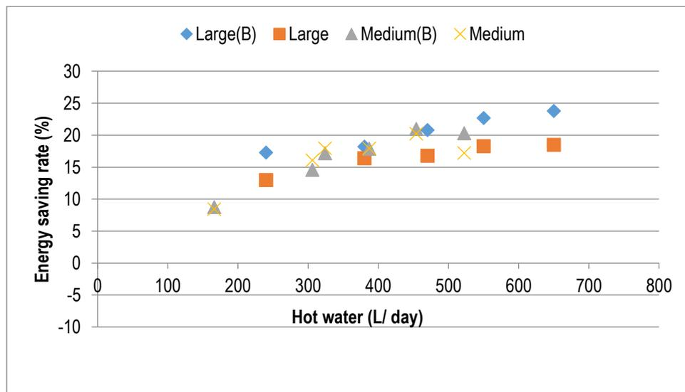
Figure 10: Energy-saving rates (SOFC + battery vs SOFC)
