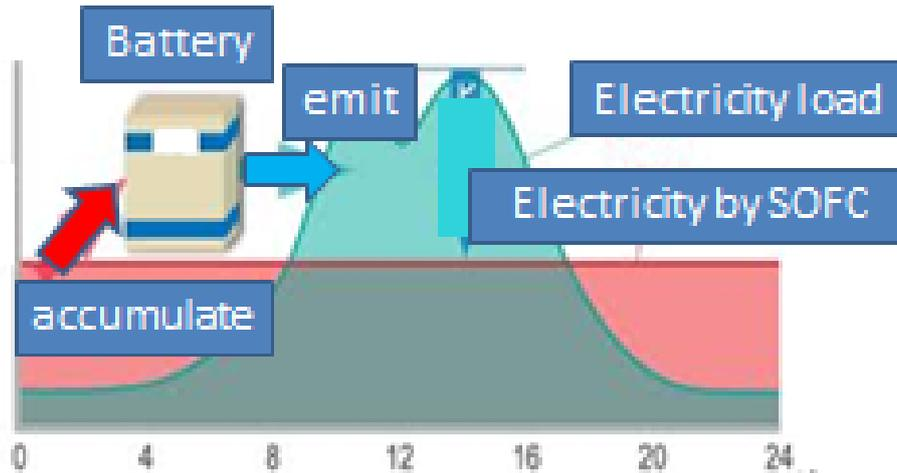
Figure 2: Operation of SOFC and battery
