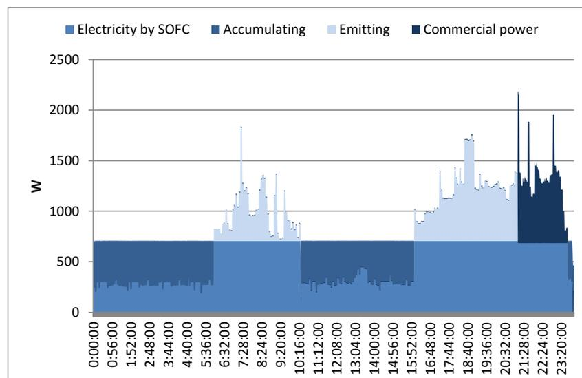
Figure 5: Supply of electric power (large 2peaks)
