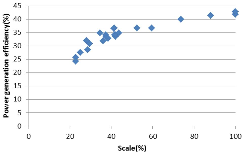
Figure 1: Power generating efficiency of SOFC
