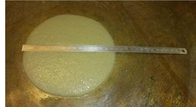
Flow test on shaking table
