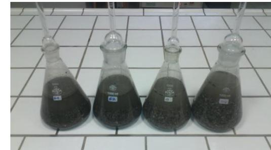
Water pycnometer test
