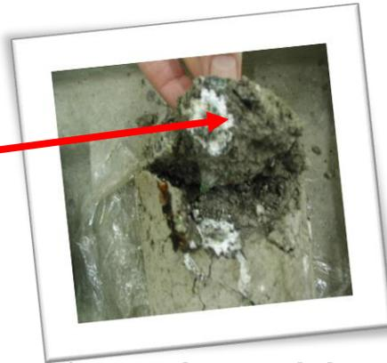
Formation of gel from oxidation of metallic aluminium
