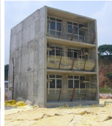
Scenario 5 – Polymethyl methacrylate (PMMA) parapet with gap
